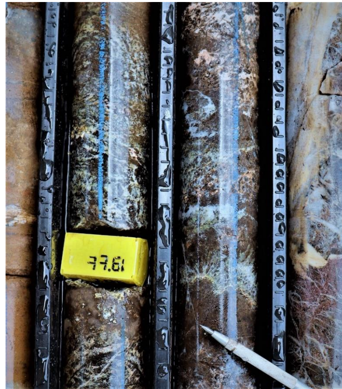
Extensive pale green monazite seen in drill core. Yellow marker is 77.61m down hole.
