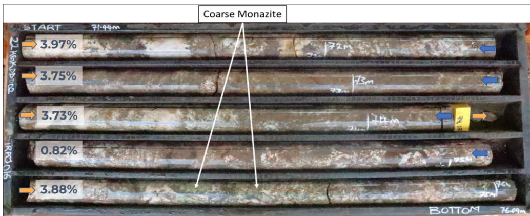
Image 1: Carbonatite with green coarse monazite mineralisation visible. Interval of KGKDD002 from 71.44m to 76.09m showing TREO%
