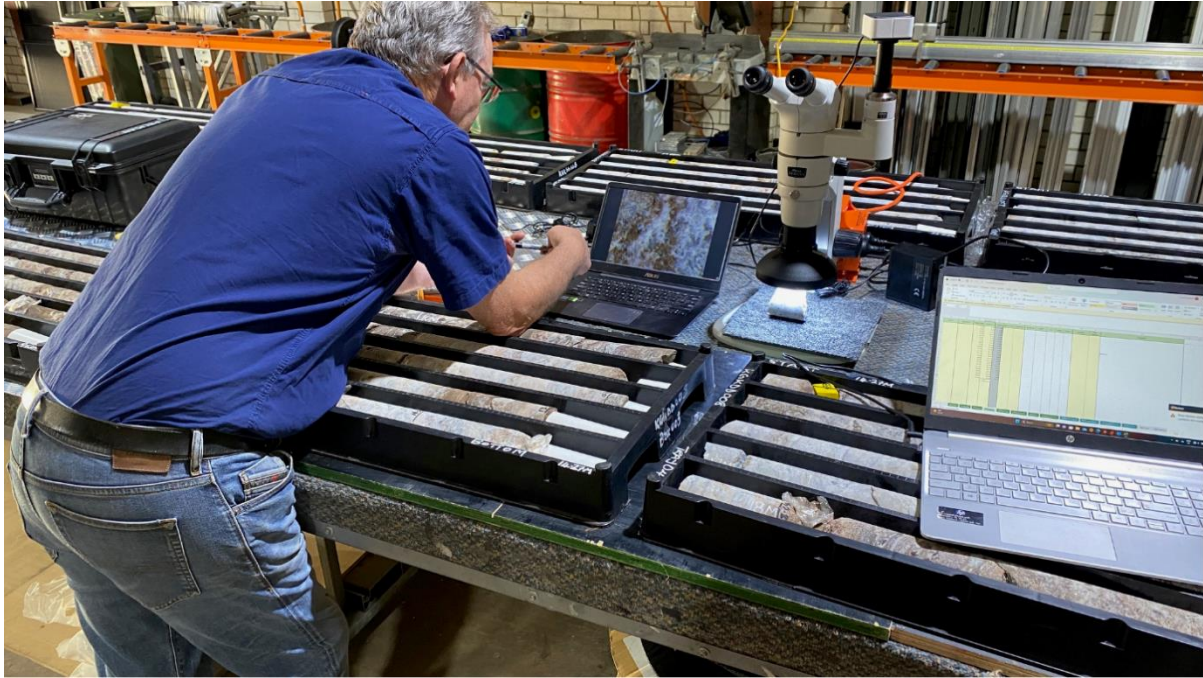
Image 8: Mineralogical Inspection of Kangankunde drill core used in metallurgical testwork.
