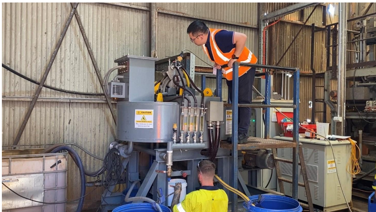
Image 5: Pilot-scale WHIMS Testing at Nagrom Laboratory in Perth, Australia
